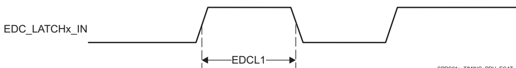
图 5-69. PRU-ICSS ECAT LATCHx_IN Timing
