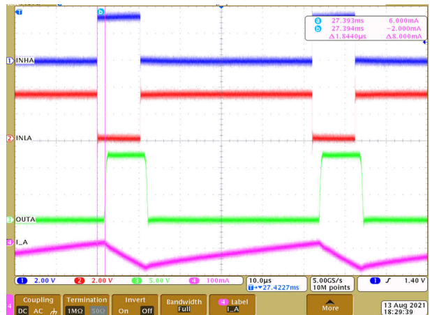
9-9. Driver delay compensation (1.8 μs)
