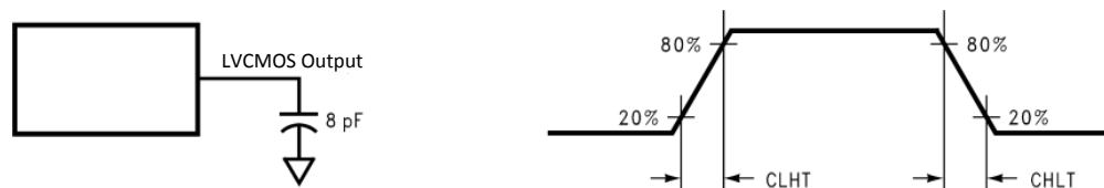
Figure 2. LVC MOS Output Load and Transition Times
