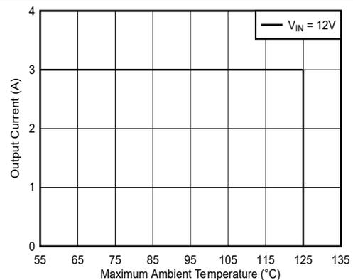
$V_{OUT} = 5V$   $F_{SW} = 400kHz$   $I_{OUT} = 3A$
