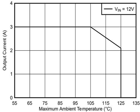
$V_{OUT} = 5V$        $F_{SW} = 2MHz$        $I_{OUT} = 3A$
