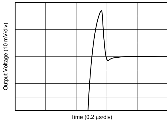
7-31. Small-Signal Step Response
