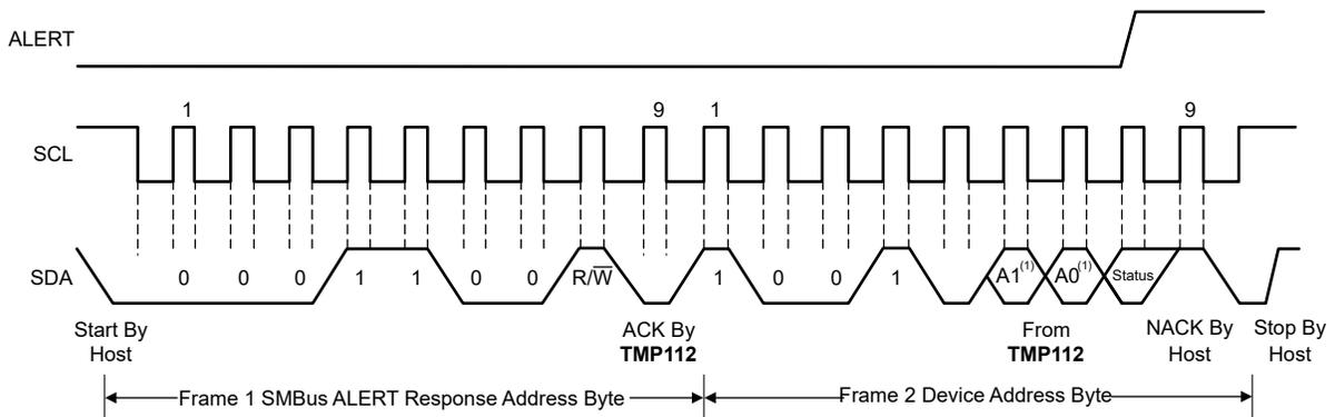
NOTE: (1) The value of A0 and A1 are determined by the ADD0 pin.
