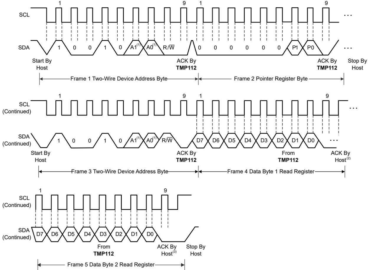
NOTE: (1) The value of A0 and A1 are determined by the ADD0 pin.
