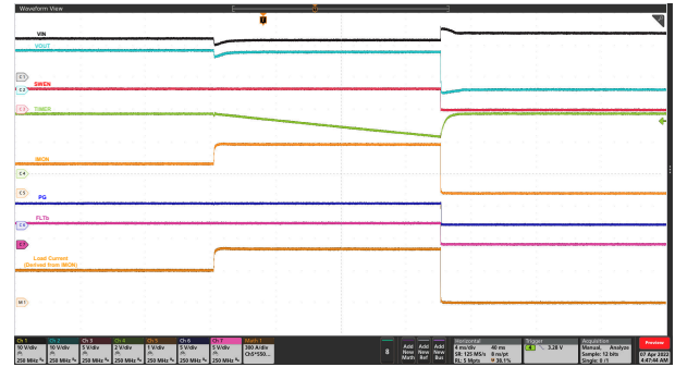
9-11. Circuit-Breaker Response: V_{IN} = 12\text{ V} , C_{ITIMER} = 22\text{ nF} , C_{LOAD} = 55\text{ mF} , R_{IMON} = 167\ \Omega , R_{IREF} = 40.2\text{ k}\Omega , and Load Current Stepped up From 300 A to 500 A for > 20 ms
