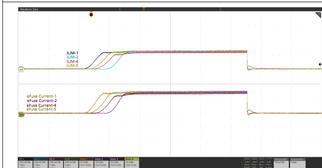
9-8. Power Up into Short (Current distribution among five devices in parallel): V_{IN} = 12 V, EN/UVLO Stepped Up From 0 V to 3 V, R_{IREF} = 40.2 k \Omega , R_{ILIM} on Each Device = 300 \Omega , and OUT Shorted to GND
