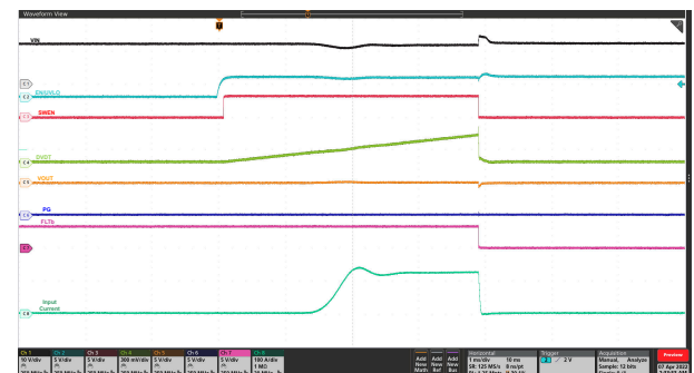
9-7. Power Up into Short: V_{IN} = 12 V, EN/UVLO Stepped Up From 0 V to 3 V, R_{IREF} = 40.2 k \Omega , R_{ILIM} on Each Device = 300 \Omega , and OUT Shorted to GND
