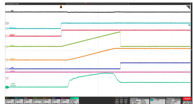
9-5. Start-up with EN/UVLO: V_{IN} = 12 V, EN/UVLO Stepped Up From 0 V to 3 V, C_{LOAD} = 55 mF, R_{LOAD(Start-up)} = 0.33 \Omega , C_{DVDT} = 33 nF, R_{IREF} = 40.2 k \Omega , and R_{ILIM} on Each Device = 300 \Omega
