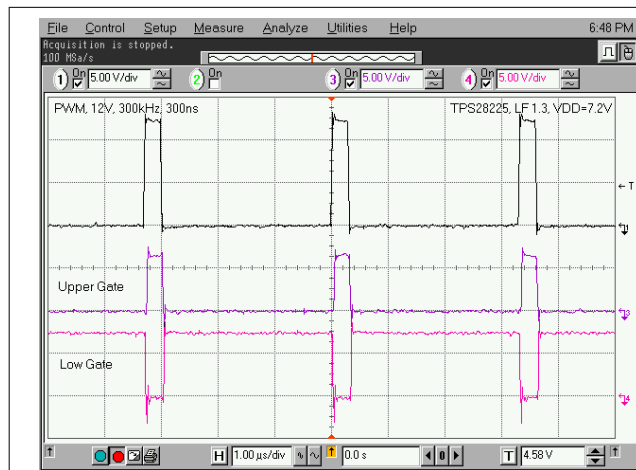
Figure 6-4. 12-V PWM Pulse at V_{DD} = 7.2\text{ V}
