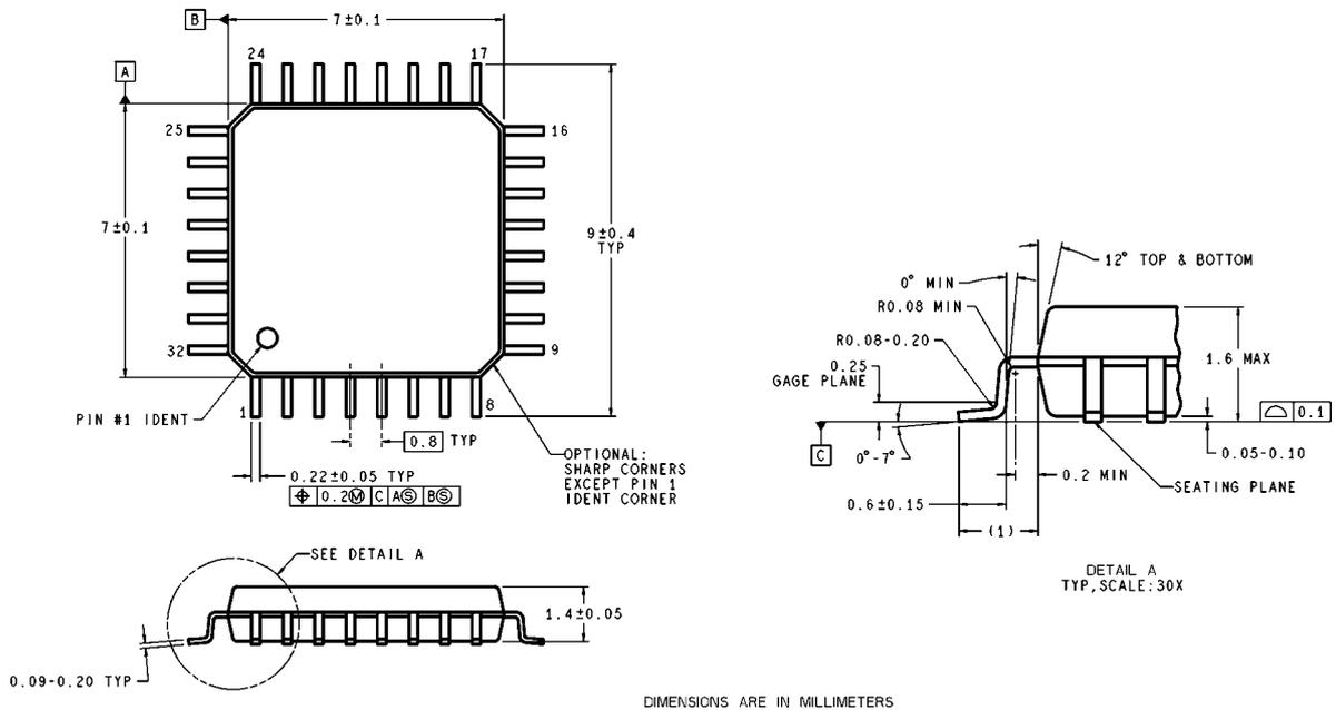
DIMENSIONS ARE IN MILLIMETERS
