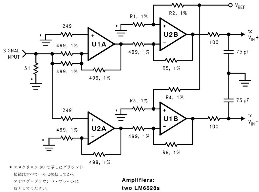
FIGURE 5. Differential Drive Circuit of FIGURE
