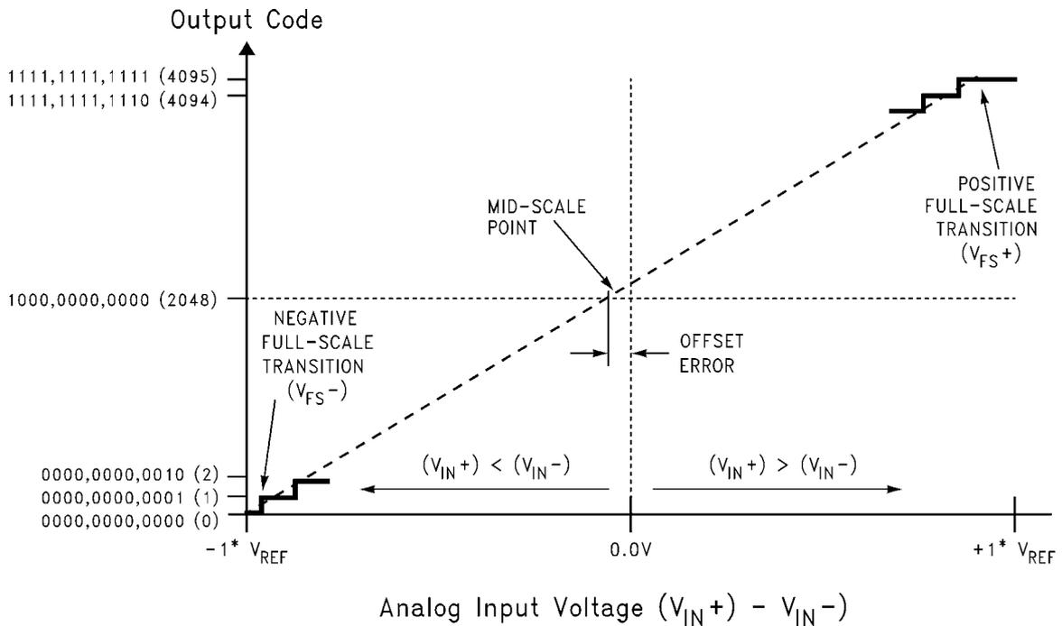
FIGURE 1. Transfer Characteristic
