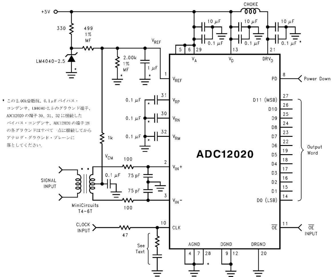
FIGURE 6. Driving the Signal Inputs with a Transformer
