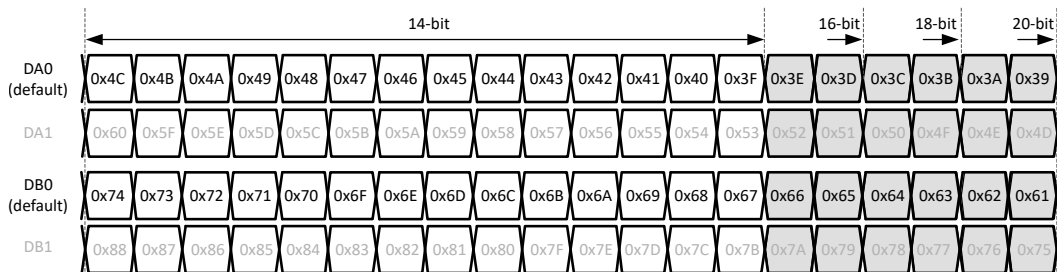
8-46. 1-wire output bit mapping
