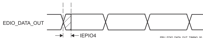
图 6-54. PRU-ICSS IEP Digital IOs Timing Requirements
