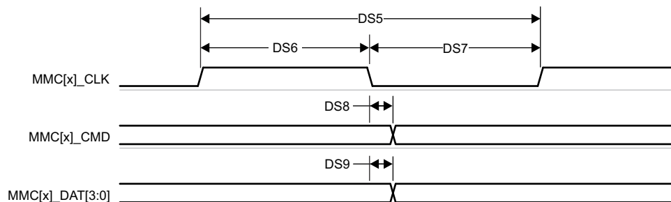
図 6-84. MMC1/MMC2 – Default Speed – Transmit Mode
