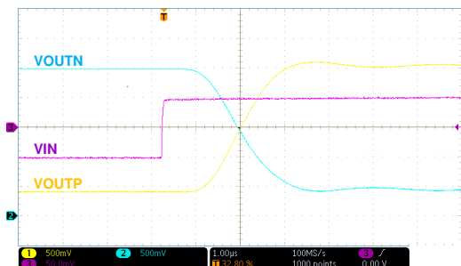
Figure 8-4. Step Response of the AMC1202
