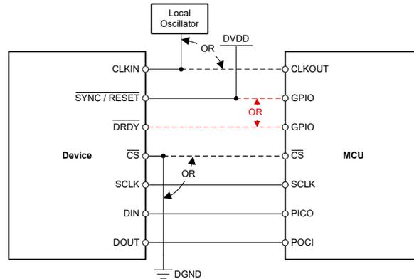
**図 9-2. Minimum Connections Required to Operate the AMC131M03**
