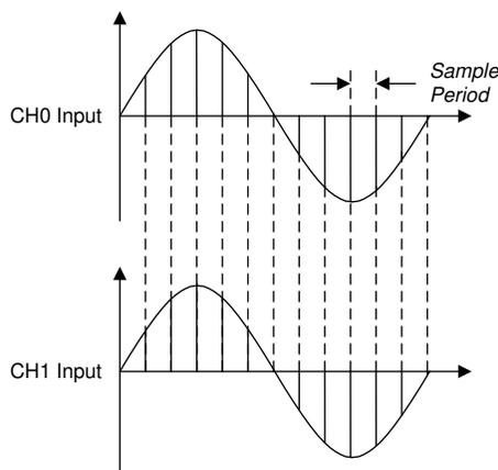
**Figure 8-11. Two Channel Outputs With Equal Phase Settings**
