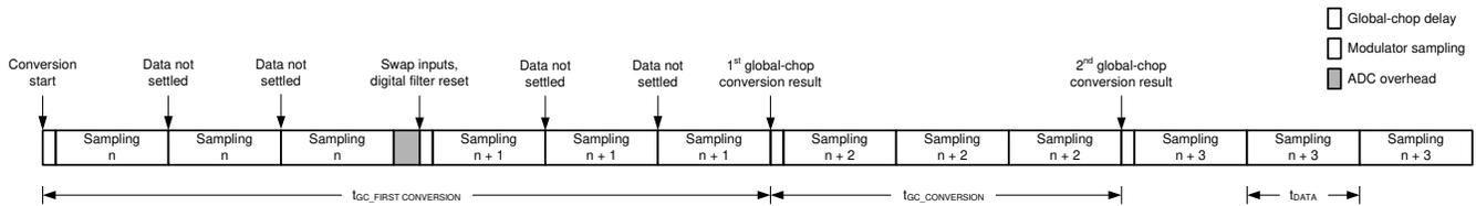
Figure 8-23. Conversion Timing With Global-Chop Mode Enabled
