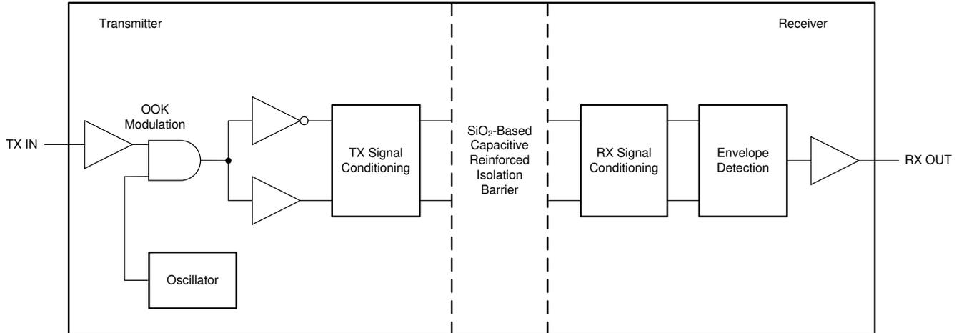
**図 8-1. Block Diagram of an Isolation Channel**
