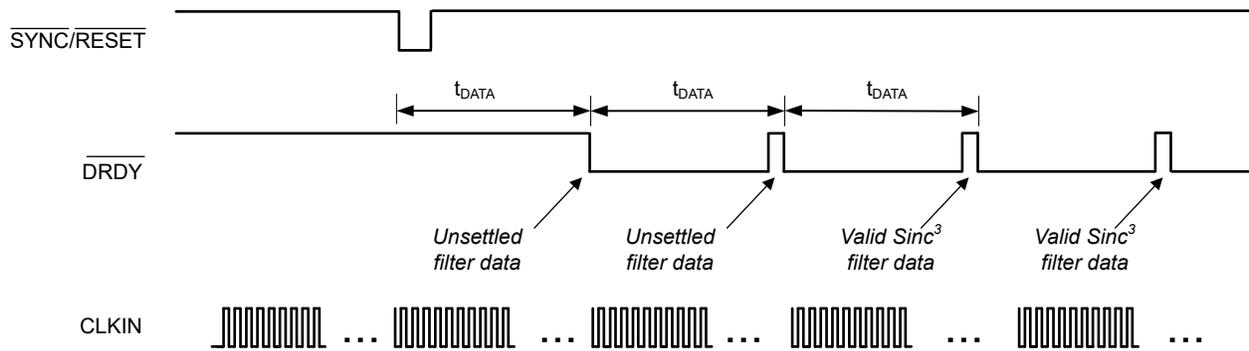
Figure 8-21. Synchronization Timing for OSR = 1024
