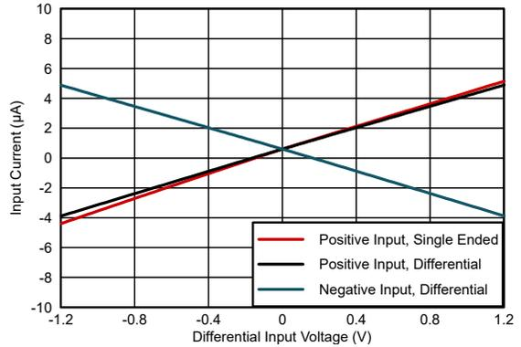
图 6-7. Input Current vs Differential Input Voltage
