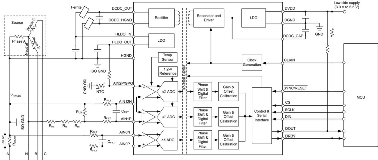
図 9-5. Current and Voltage Sensing With the AMC131M03
