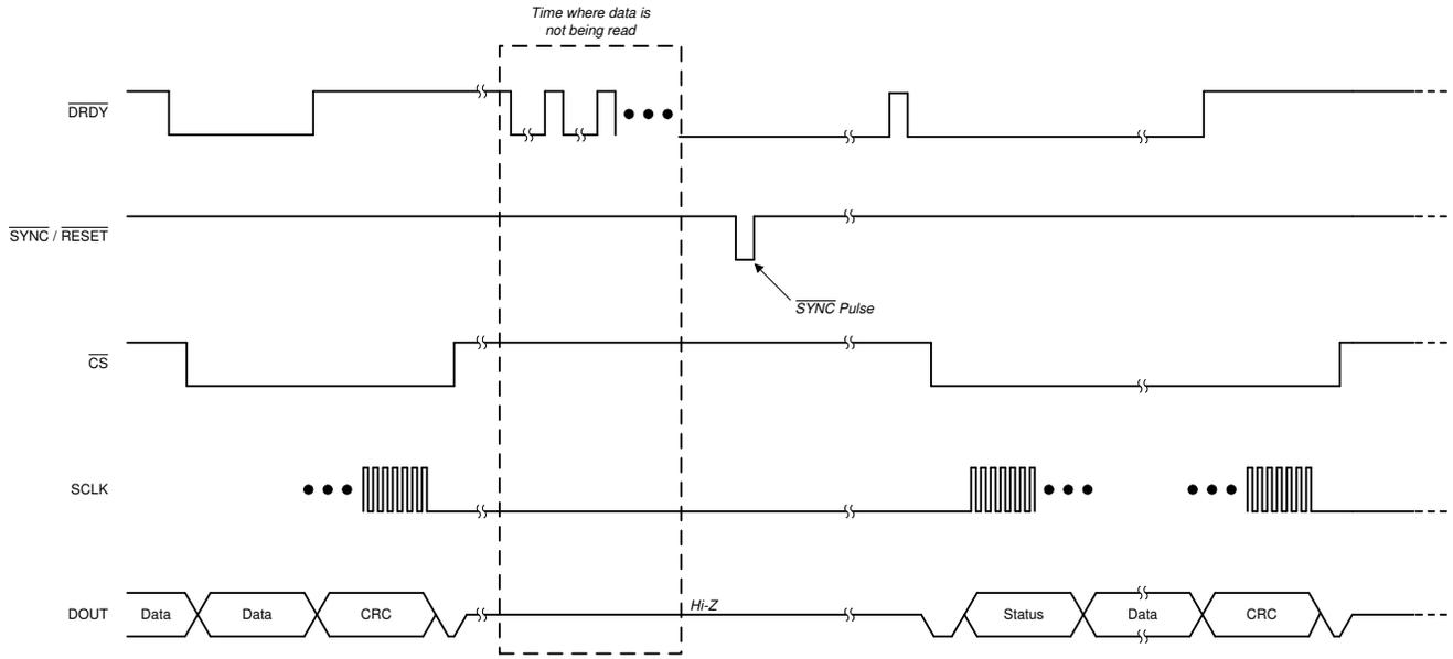
8-31. Collecting Data After a Pause Using the  $\overline{\text{SYNC/RESET}}$  Pin
