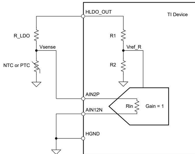
8-16. External Temperature Sensor Measurement Block Diagram
