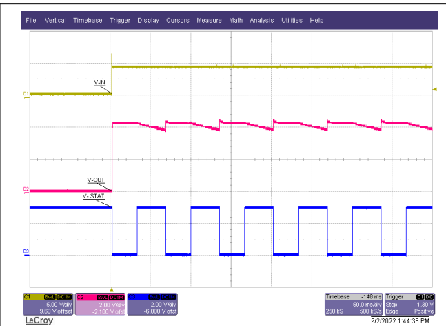
図 8-3. Power Up Without Battery
