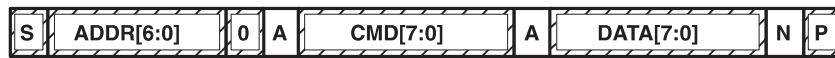
Figure 6. Attempt To Write a Read-only Address (Nack After Data Sent By Master)
