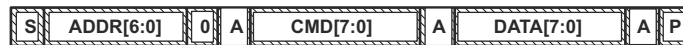
Figure 7-2. Attempt To Write a Read-Only Address (Nack After Data Sent By Master)
