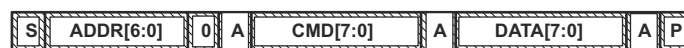
7-3. Attempt To Write a Read-Only Address (Nack After Data Sent By Master)
