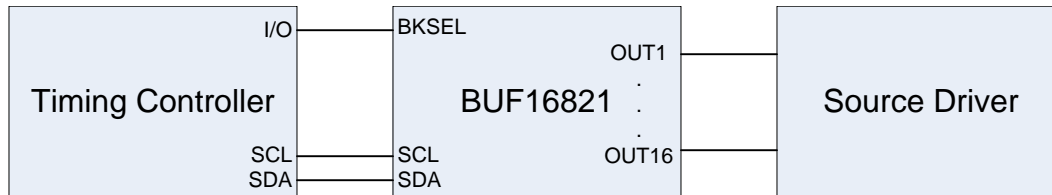
Figure 20. Gamma Control Block Diagram
