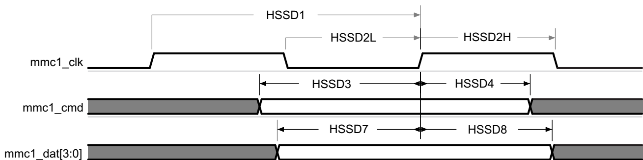
图 7-64. MMC/SD/SDIO in - High Speed - Receiver Mode
