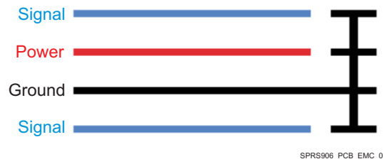
Figure 8-13. Guard Ring Routing
