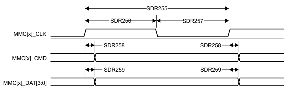
図 6-104. MMC1/2 – UHS-I SDR25 – Transmit Mode
