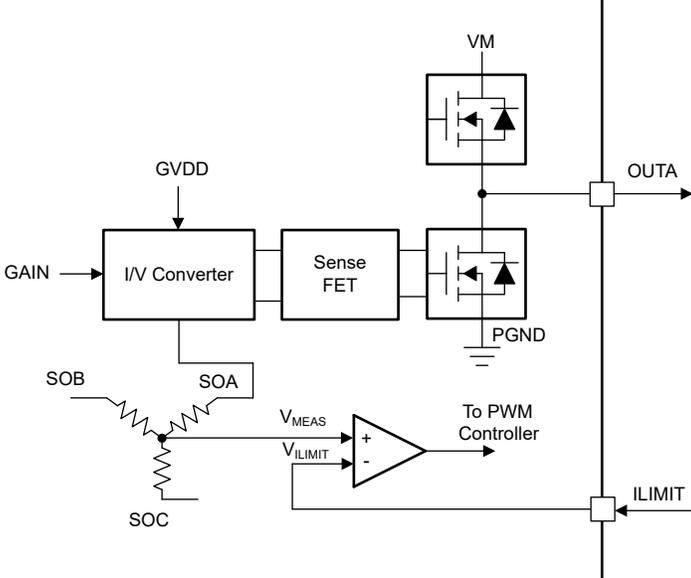
shows the implementation of current limit circuitry, the output of current sense amplifiers are combined with star connected resistive network. This measured voltage  $V_{MEAS}$  is compared with the external reference voltage  $V_{ILIMIT}$  pin to realize the current limit implementation. The relation between current sensed on OUTX pin and  $V_{MEAS}$  threshold is given as:
