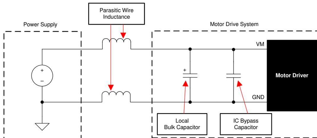
图 8-2. Example Setup of Motor Drive System With External Power Supply
