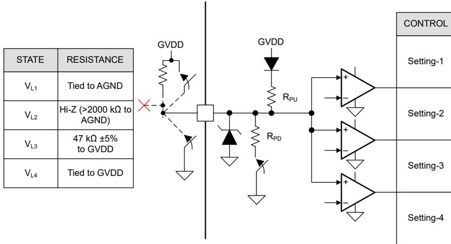
7-19. Four Level Input Pin Structure
