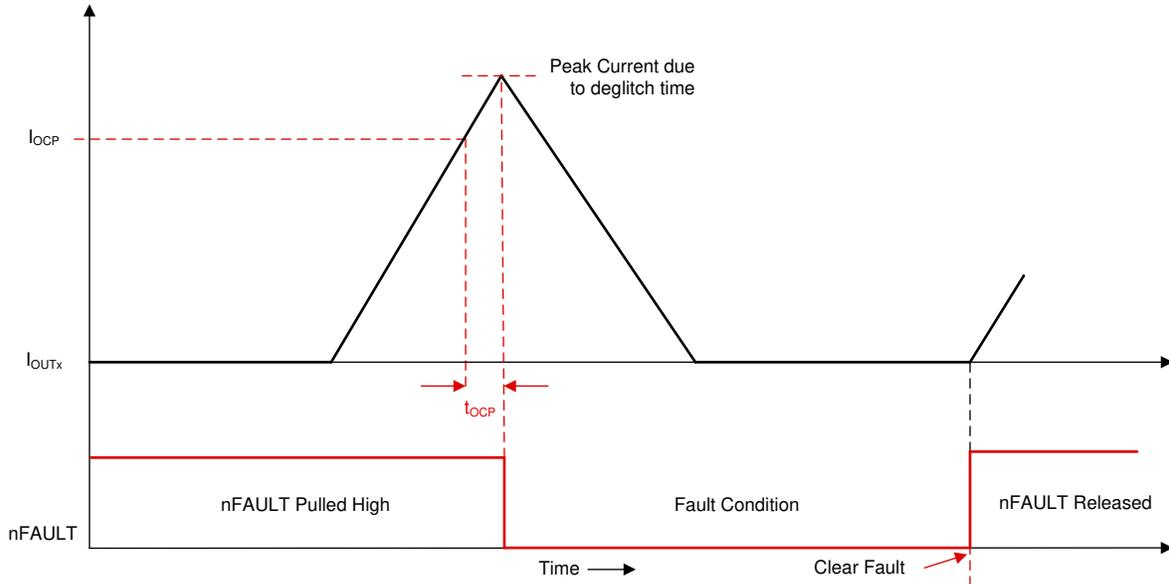
图 7-37. Overcurrent Protection - Latched Shutdown Mode
