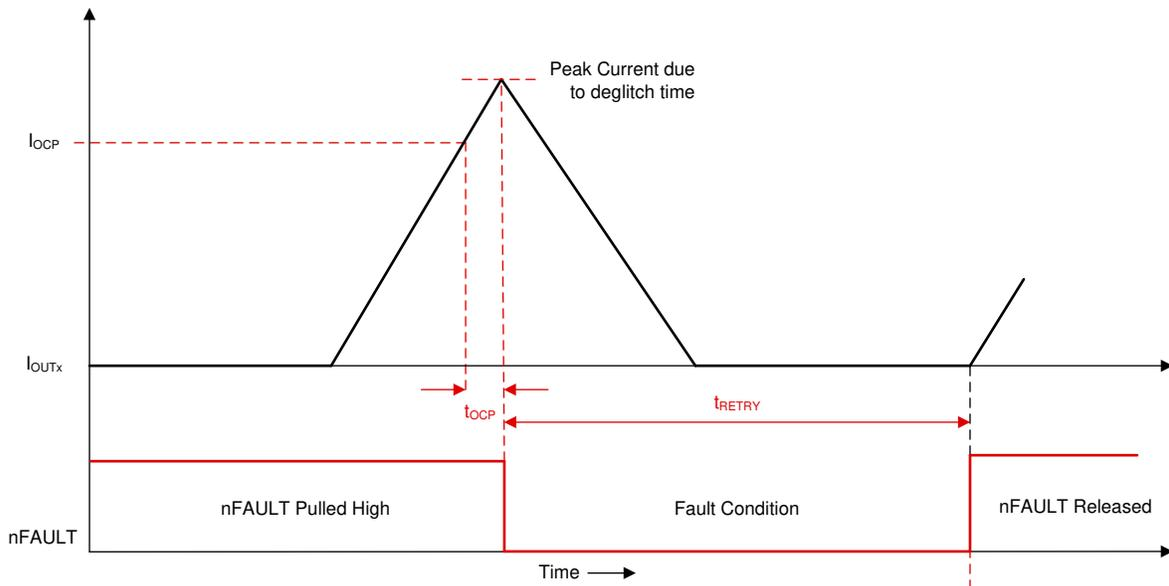
图 7-38. Overcurrent Protection - Automatic Retry Mode
