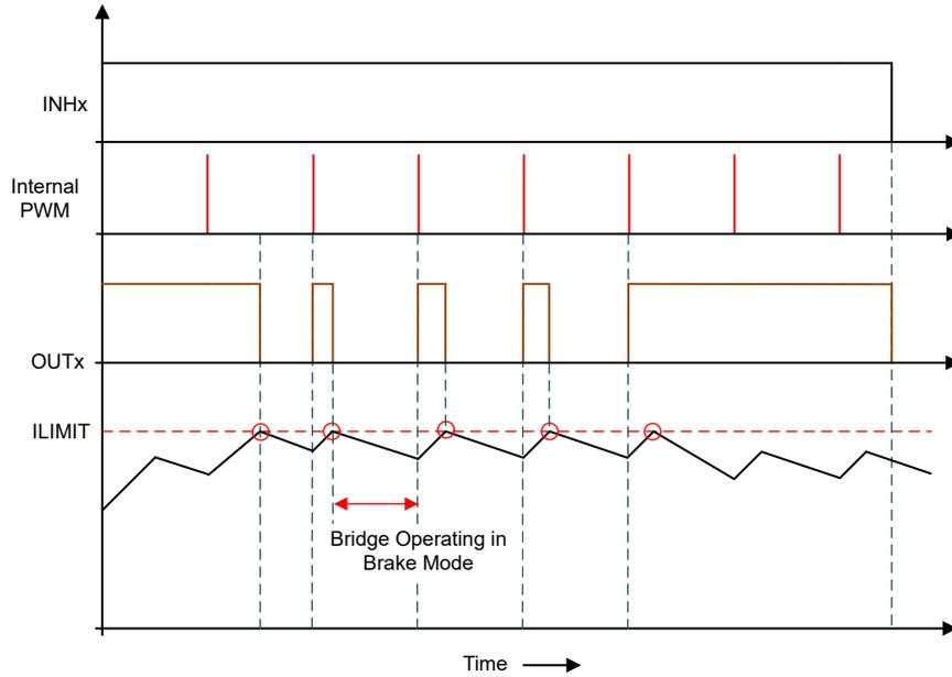
图 7-34. Cycle-by-Cycle Current-Limit Operation with 100% PWM Duty Cycle
