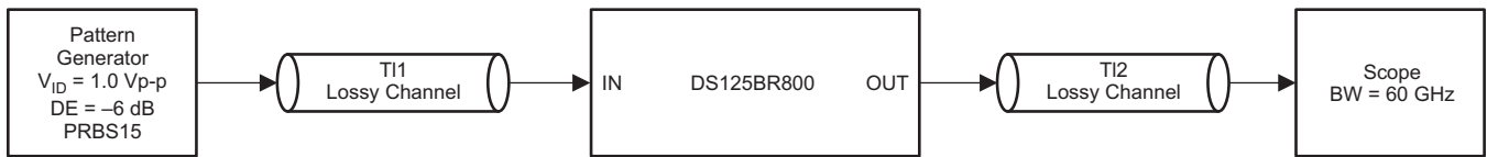
Figure 11. Test Setup Connections Diagram
