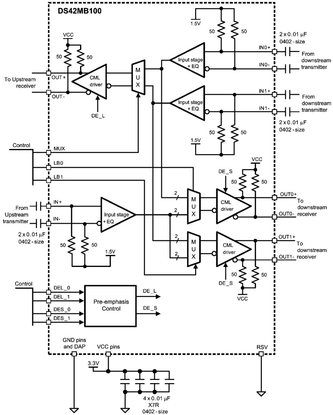
FIGURE 7. Application Diagram
