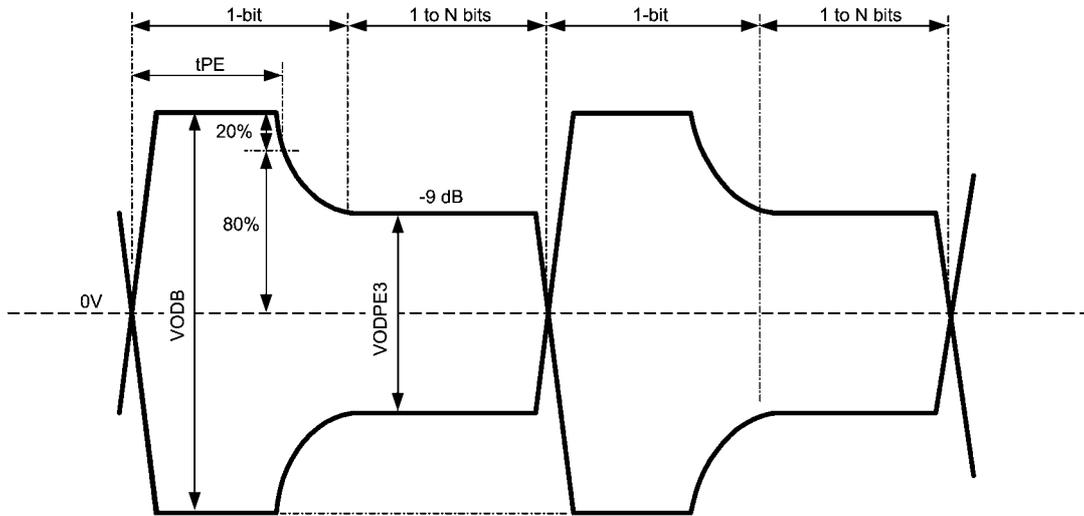
FIGURE 4. Test Condition For Output Pre-Emphasis Duration
