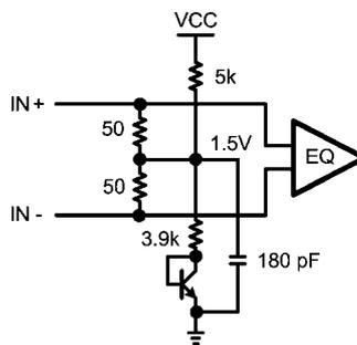
FIGURE 6. Receiver Input Termination and Bias Circuit
