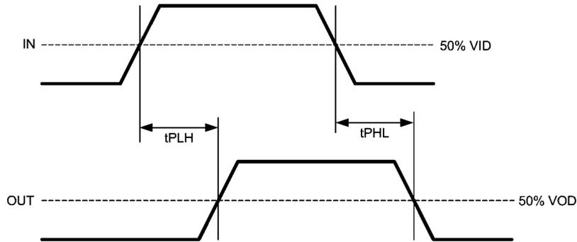
**FIGURE 3. Propagation Delay From Input To Output**
