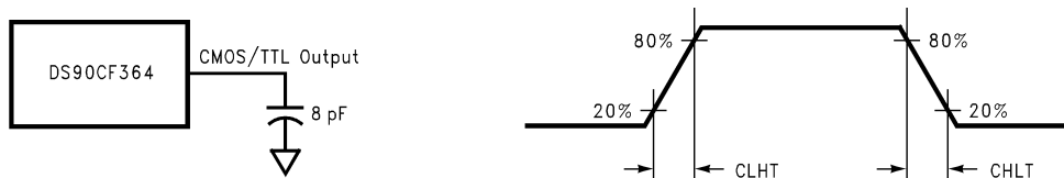
FIGURE 4. DS90CF364 (Receiver) CMOS/TTL Output Load and Transition Times
