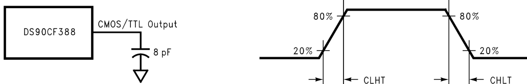
FIGURE 4. DS90CF388 (Receiver) CMOS/TTL Output Load and Transition Times
