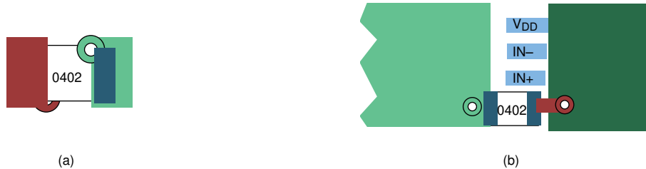
Figure 11-7. Typical Decoupling Capacitor Layouts
