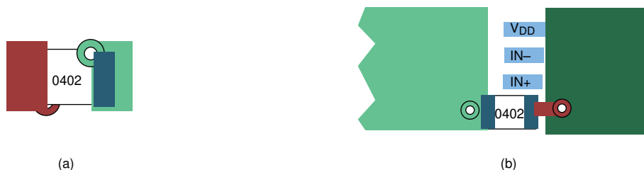
Figure 21. Typical Decoupling Capacitor Layouts
