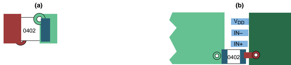
Figure 18. Typical Decoupling Capacitor Layouts
