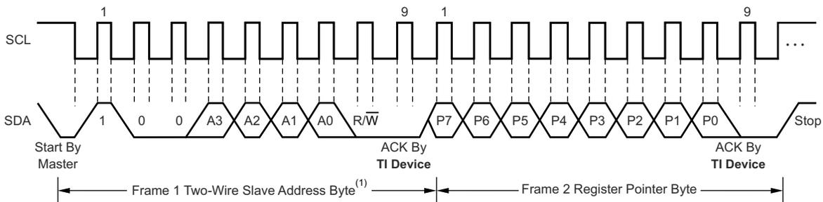
A. The slave address byte value is determined by the settings of the A0 and A1 pins. Refer to [表 8-2](#).
