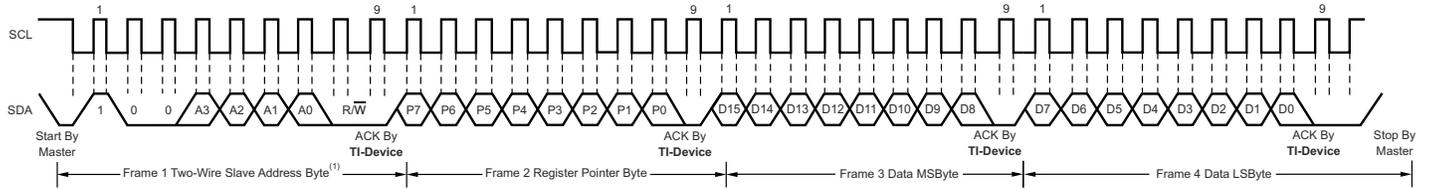
A. The value of the slave address byte is determined by the settings of the A0 and A1 pins. Refer to [表 8-2](#).
