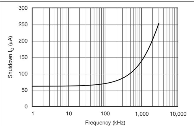
**7-19. Shutdown  $I_Q$  vs  $I^2C$  Clock Frequency**
