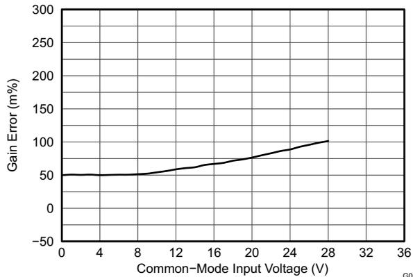
**7-8. Shunt Input Gain Error vs Common-Mode Voltage**
