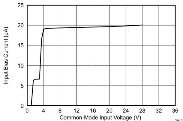
**7-13. Input Bias Current vs Common-Mode Voltage**
