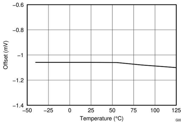
**7-10. Bus Input Offset Voltage vs Temperature**
