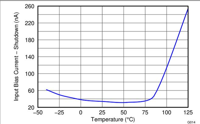
**7-15. Input Bias Current vs Temperature, Shutdown**
