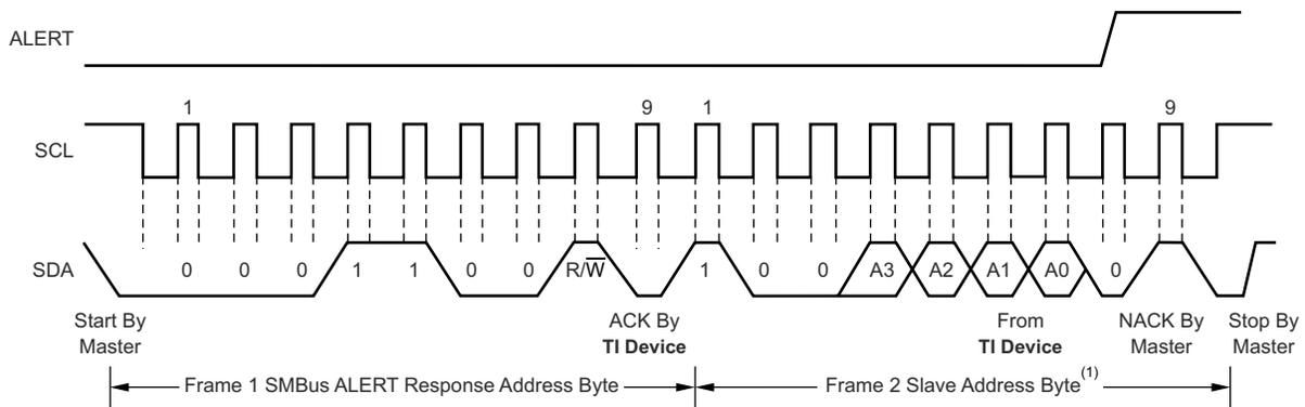
A. The slave address byte value is determined by the settings of the A0 and A1 pins. Refer to [表 8-2](#).
