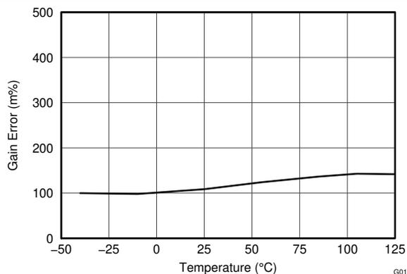
**7-12. Bus Input Gain Error vs Temperature**
