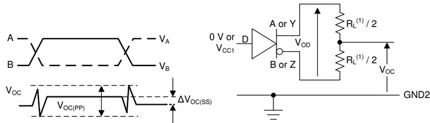
A.  $R_L = 100\Omega$  (RS422)、 $R_L = 54\Omega$  (RS-485)
