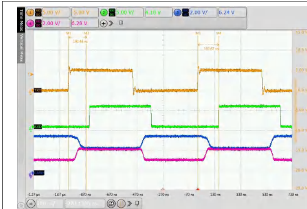
8-15. Typical TXD, RXD, CANH and CANL Waveforms at 2 Mbps
