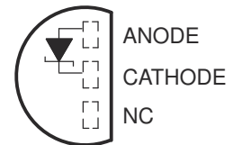
1.2 V ... LP (TO-92/TO-226) PACKAGE (TOP VIEW)
