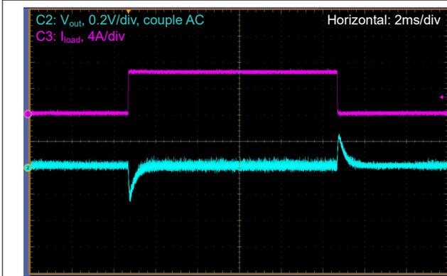
7-16. Load Transient,  $V_{in} = 14.4V$ ,  $V_{out} = 24V$ , FPWM,  $I_{load} = 0A$  to  $6.25A$  at  $1A/\mu s$
