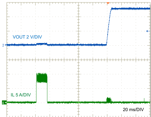
8-10. LM634x0-Q1 Short-Circuit Recovery to No Load
