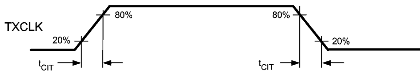
FIGURE 2. Transmit Clock Transition Times
