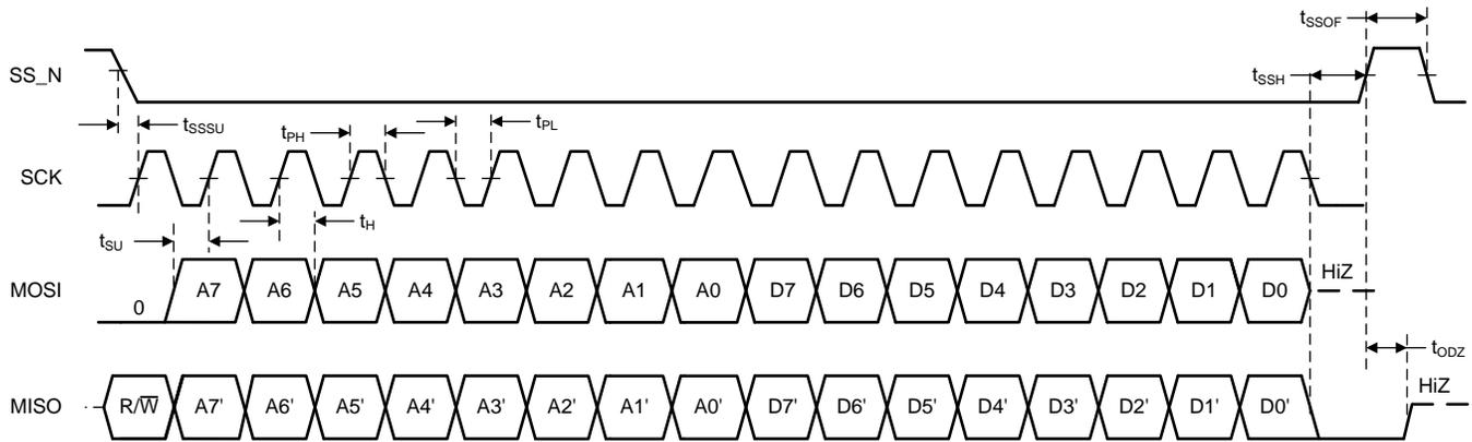
**Figure 18. Signal Timing for a SPI Write Transaction**
