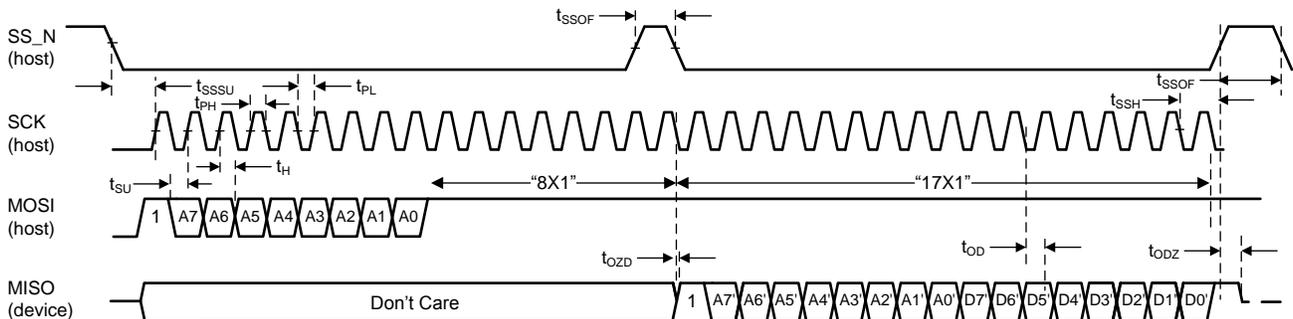
**Figure 19. Signal Timing for a SPI Read Transaction**
