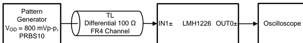
22. Test Setup for LMH1226 PCB Equalizer (IN1±)
