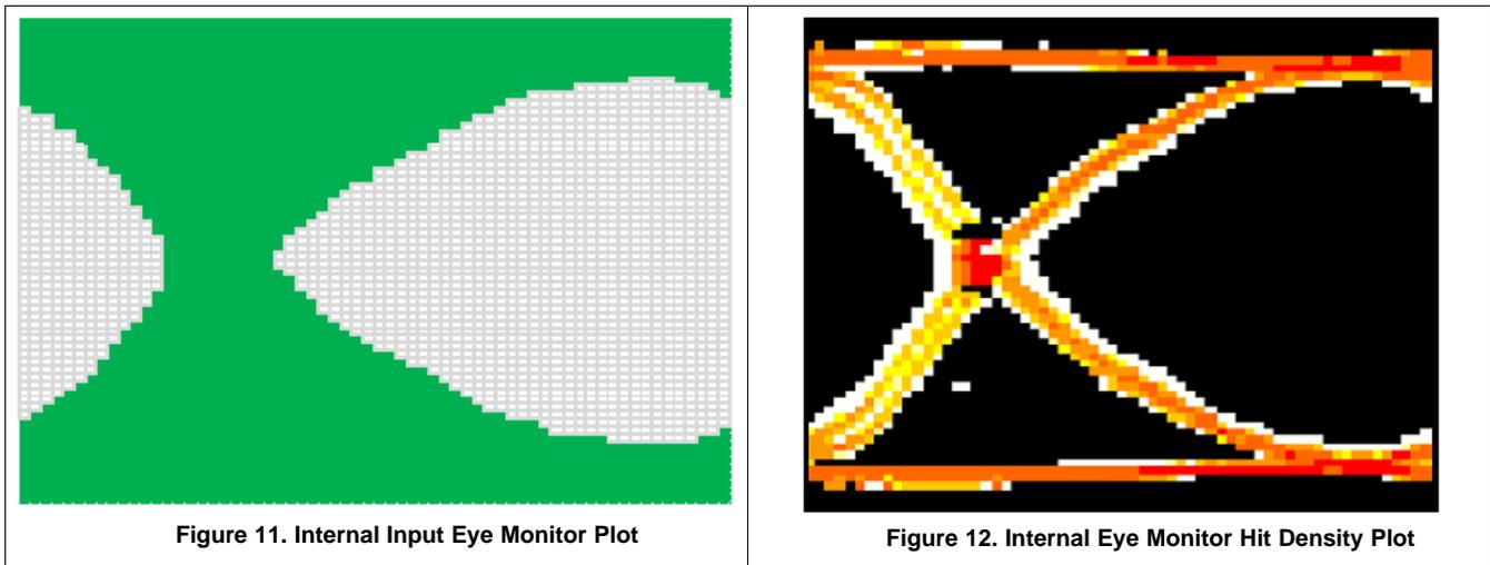
Figure 11. Internal Input Eye Monitor Plot
