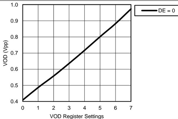
Figure 9. VOD vs. VOD and DEM Register Settings
