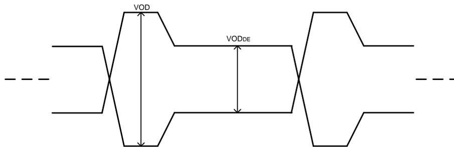
**Figure 13. VOD and VOD<sub>DE</sub> Levels**
