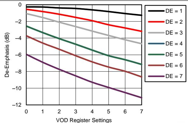
Figure 10. De-Emphasis vs. VOD and DEM Register Settings
