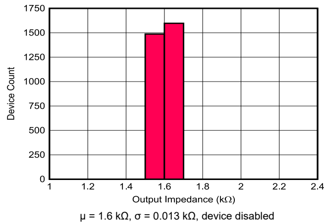
5-27. Output Impedance ( Z_{OUT} ) Distribution
