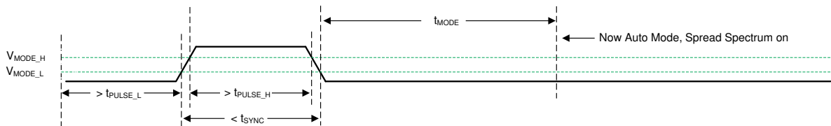
図 7-5. Transition from SYNC Mode to Auto Mode
