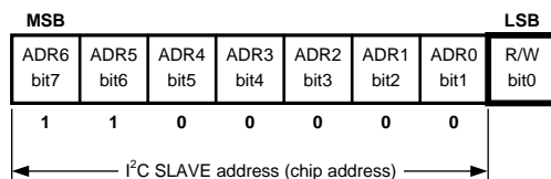
Figure 41. I 2 C Chip Address (see note above)
