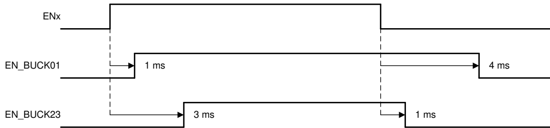
10. Typical Start-Up and Shutdown Sequencing
