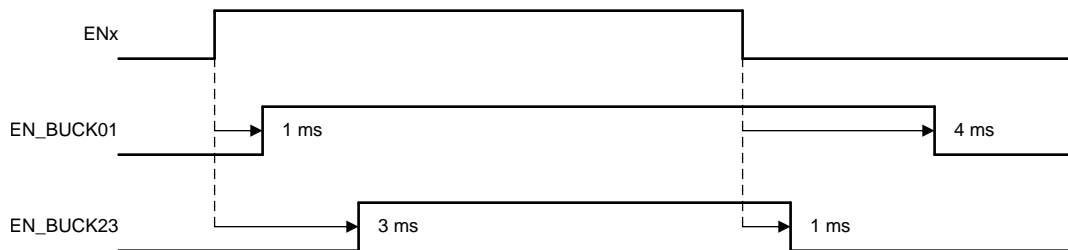
图 16. Typical Start-Up and Shutdown Sequencing
