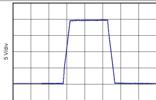
Time (50 \mu\text{s}/\text{div} ) G = -1 R_L = 10\text{ k}\Omega C_L = 10\text{ pF}
