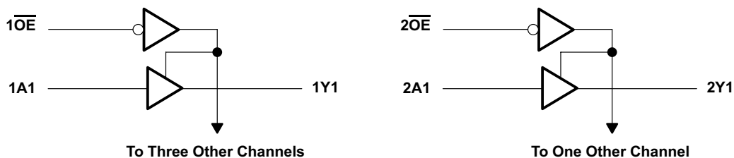
图 7-1. Logic Diagram (Positive Logic)
