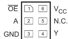
✎ 5-1. DBV package 5-pin SOT-23 (Top View)
