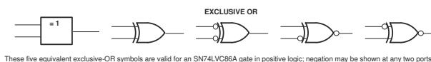
These five equivalent exclusive-OR symbols are valid for an SN74LVC86A gate in positive logic; negation may be shown at any two ports.
