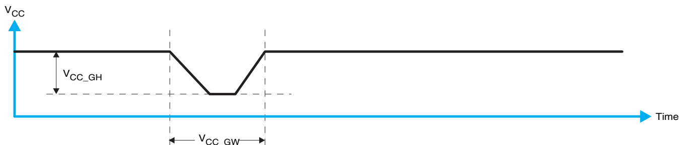
Figure 3. Glitch Width and Glitch Height
