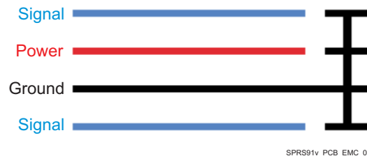
Figure 8-13. Guard Ring Routing
