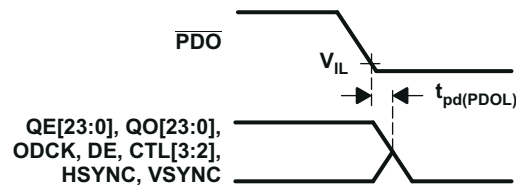
图 6-7. Delay From \overline{\text{PDO}} Low to Hi-Z Outputs
