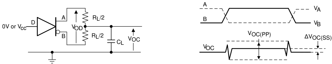
7-2. Measurement of Driver Differential and Common-Mode Output With RS-485 Load
